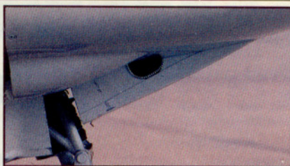
Barn-door cowl flap is electrically actuated and infinitely variable from fully open (above), for climb, to completely closed (below).
