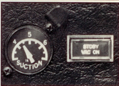
Dual vacuum pumps are standard on the 252. Annunciator warns of low vacuum pressure. Rocker switch activates standby pump.
