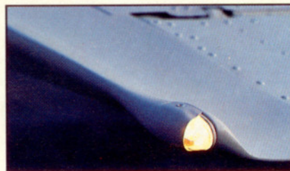
Wing-tip lighting includes highly visible recognition lights and strobes (above), plus rear-facing white position light.
