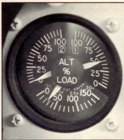
Combination gauge displays output of each alternator as well as the load or voltage on the airplane's single electrical bus.
